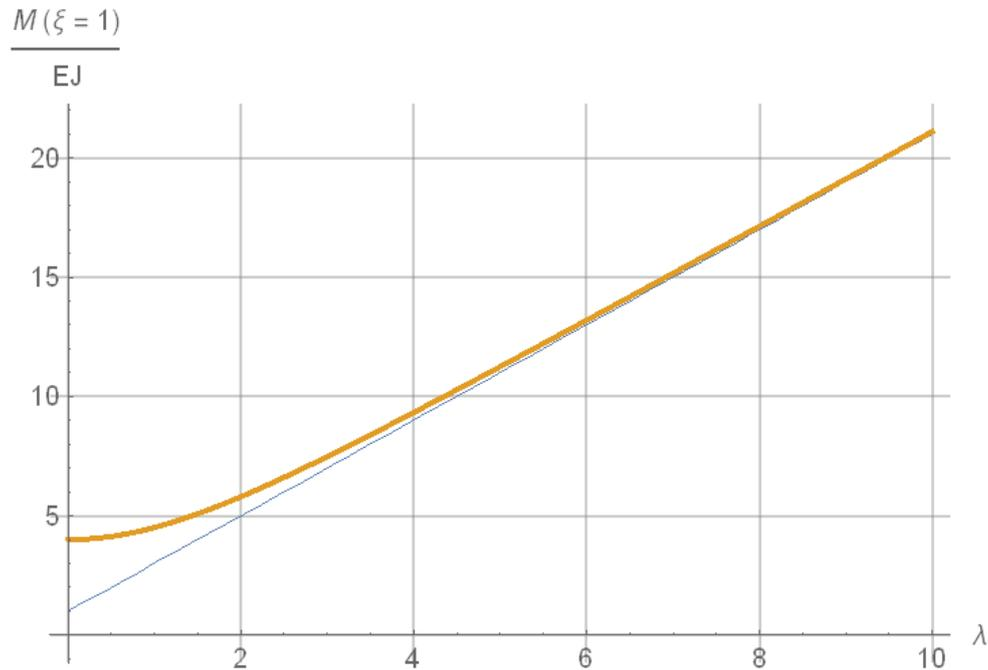
**Fig. 11.** Bending moment by the right clamp of the bar subjected to the unit rotation as function of parameter  $\lambda$
