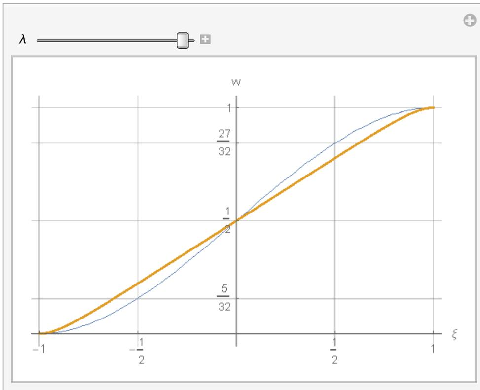
**Fig. 3. Deformation of the bar subjected to the unit transverse displacement of the right support, for  $\lambda > 0$**
