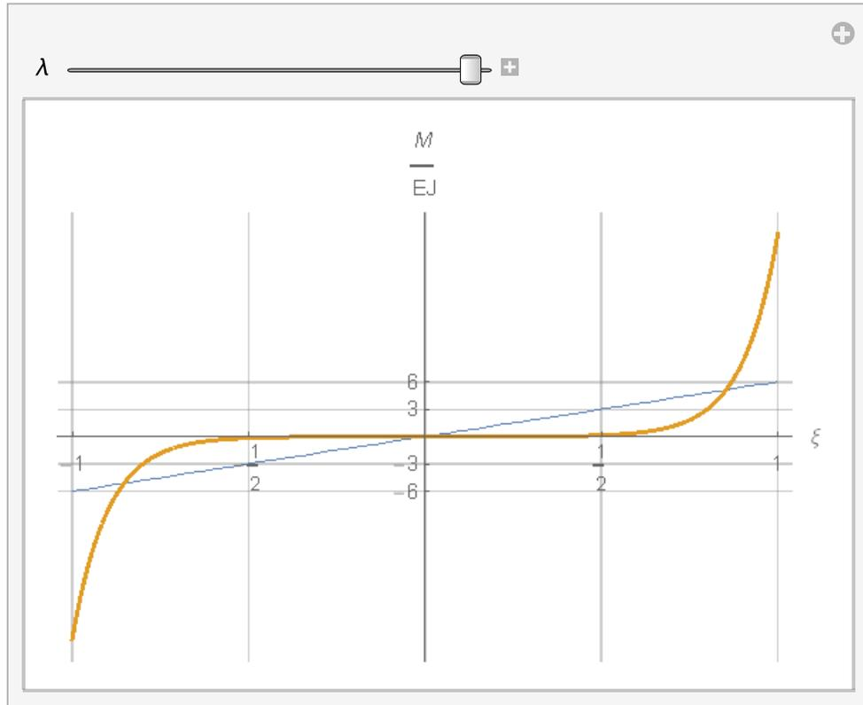
**Fig. 5. Bending moment of the bar subjected to the unit transverse displacement of the right support, for  $\lambda = 0$**
