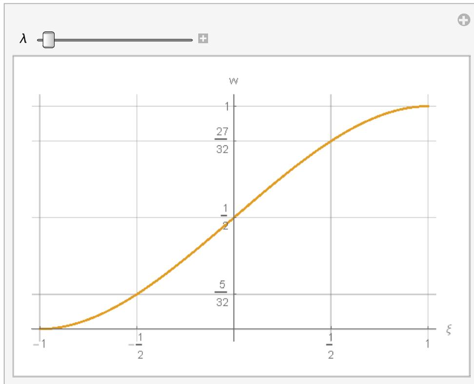
***Fig. 2. Deformation of the bar subjected to the unit transverse displacement of the right support, for  $\lambda = 0$***
