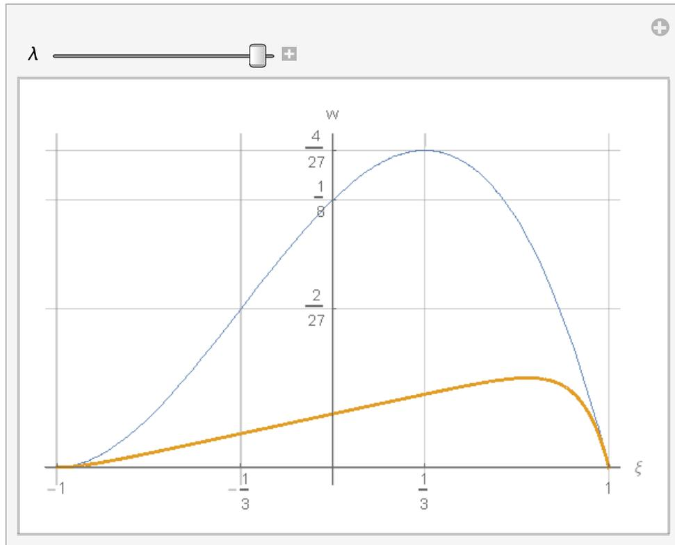
*Fig. 8. Deformation of the bar subjected to the unit rotation of the right support, for  $\lambda > 0$*
