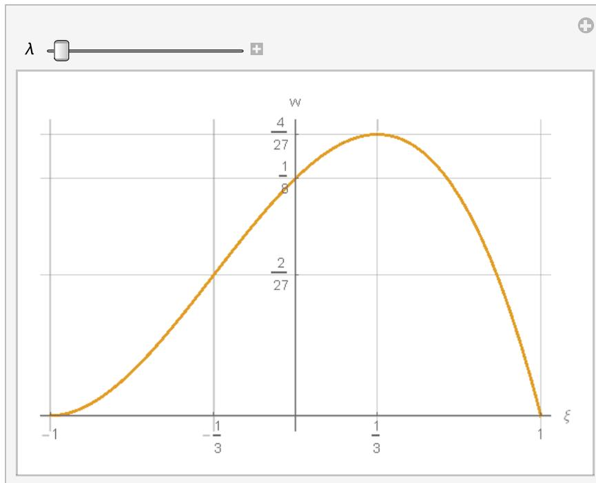
**Fig. 7. Deformation of the bar subjected to the unit rotation of the right support, for  $\lambda = 0$**
