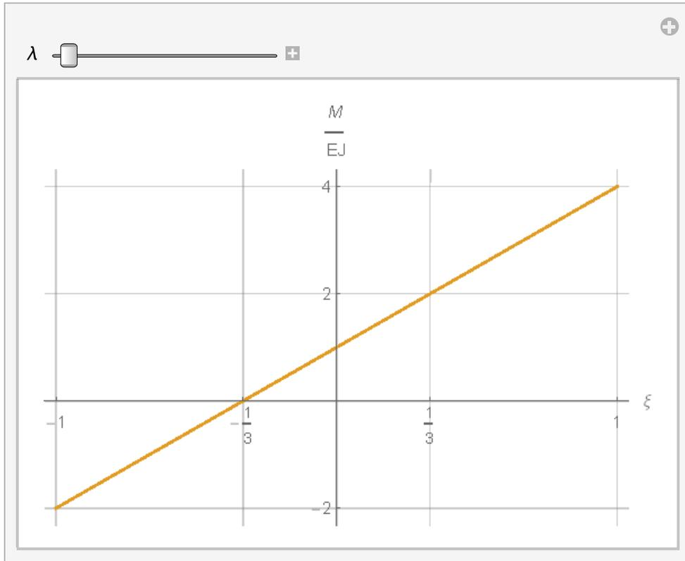
**Fig. 9. Bending moment of the bar subjected to the unit rotation of the right support, for  $\lambda = 0$**
