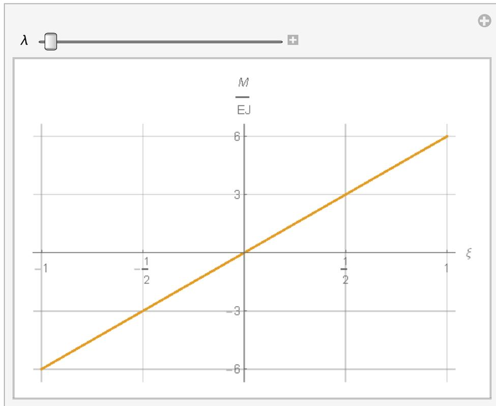
**Fig. 4. Bending moment of the bar subjected to the unit transverse displacement of the right support, for  $\lambda = 0$**
