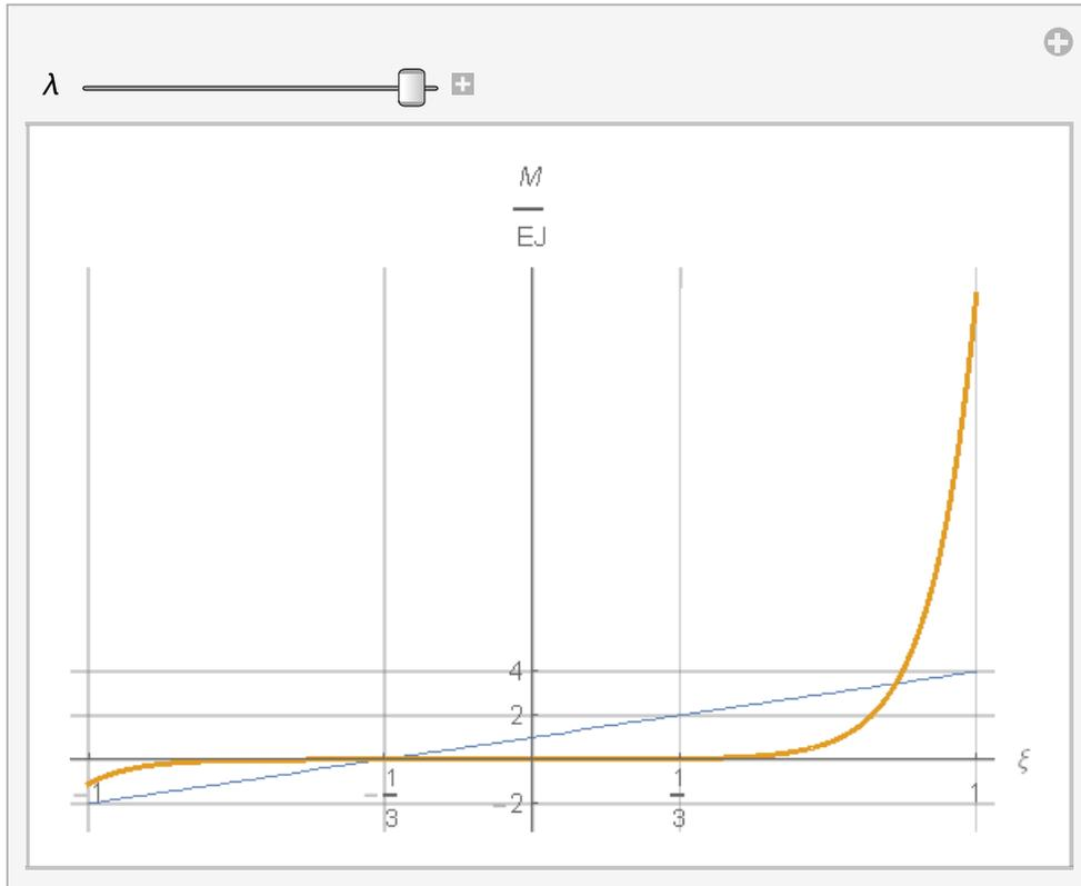
**Fig. 10. Bending moment of the bar subjected to the unit rotation of the right support, for  $\lambda > 0$**
