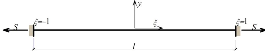
*Fig. 1. Static scheme of a clamped-clamped bar subjected to tension force*
