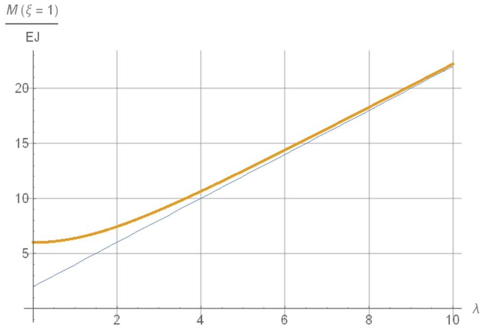
**Fig. 6. Bending moment by the right clamp of the bar subjected to the unit transverse displacement as function of parameter  $\lambda$**
