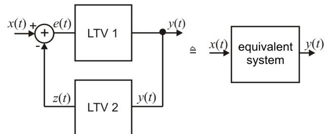
Fig. 2. Feedback system of LTV sections
