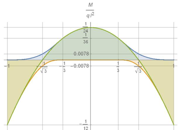
Fig. 1:  $M_g(\xi)$ ,  $M_{p+}(\xi)$ ,  $M_{p-}(\xi)$  functions for clamped-clamped beam
