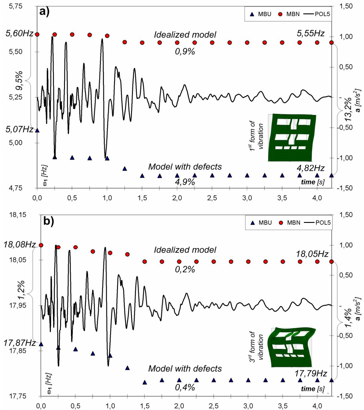
**Fig. 3** The evolution of the natural frequencies of both two walls models - MBN and MBU, depending on the kinematics excitation: a) I frequency, b) III frequency
