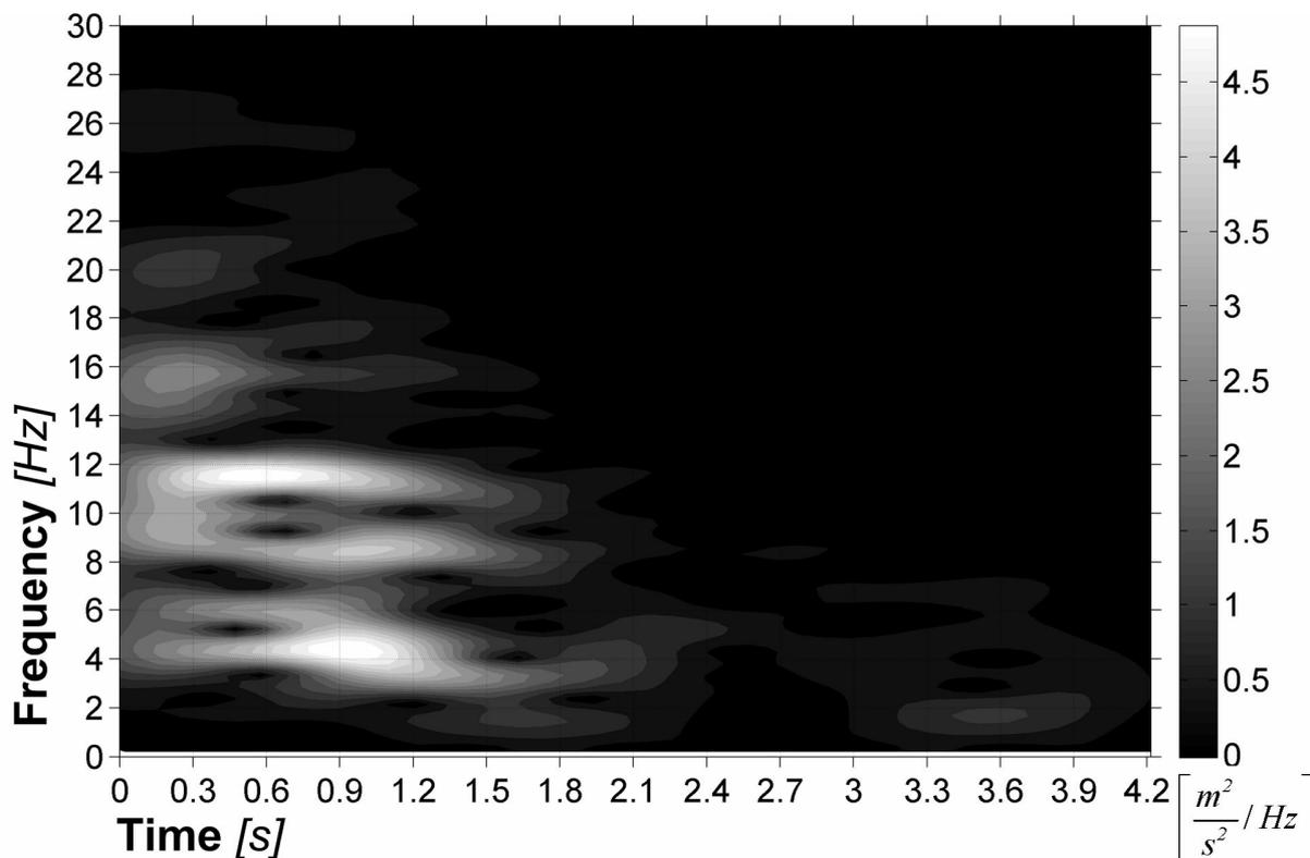
Fig. 2. Spectrum of Gabor transform modules of paraseismic quake
