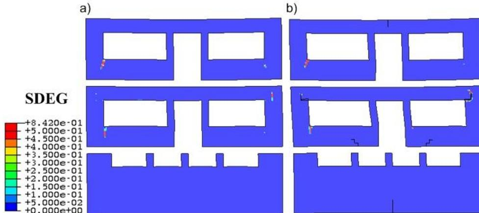
Figure 8: SDEG distribution during real enforcement: a) undamaged, b) initially damaged
