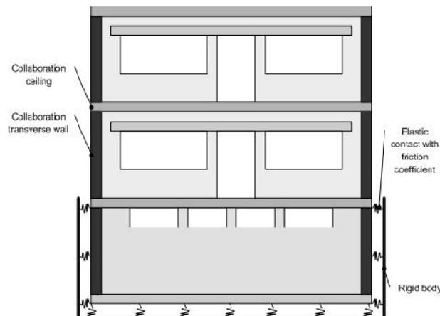
Figure 2: Details of support for the planar model
