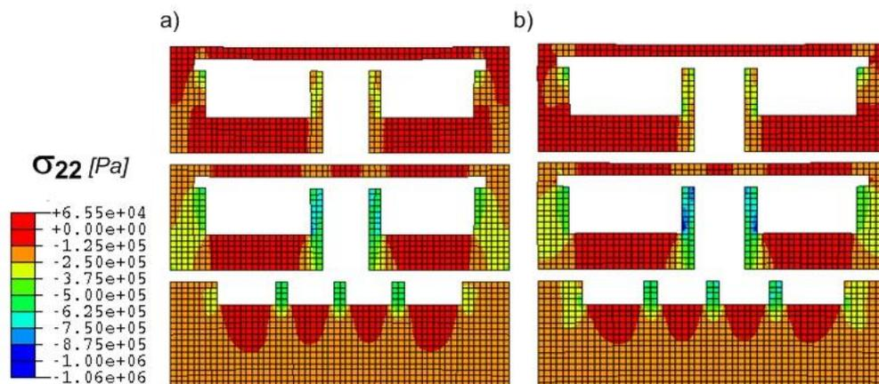
Figure 6: Vertical normal stresses distribution: a) 3D, b) 2D
