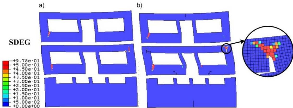
Figure 10: SDEG distribution during sin31T enforcement: a) undamaged, b) initially damaged
