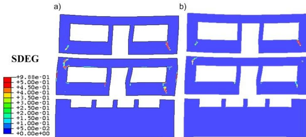
Figure 9: SDEG distribution during sin35T enforcement: a) undamaged, b) initially damaged
