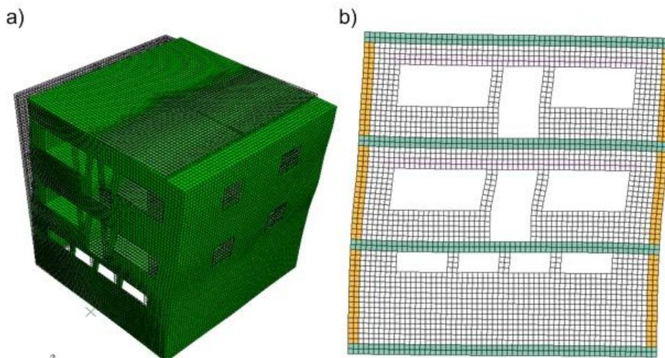
Figure 4: First form of vibration: a) 3D model, b) 2D model
