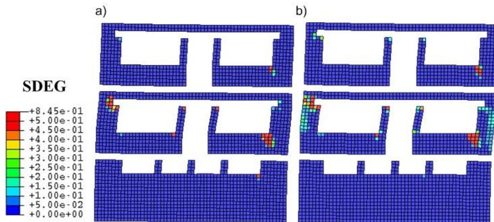
Figure 7: Distribution of the total degradation parameter: a) 3D, b) 2D
