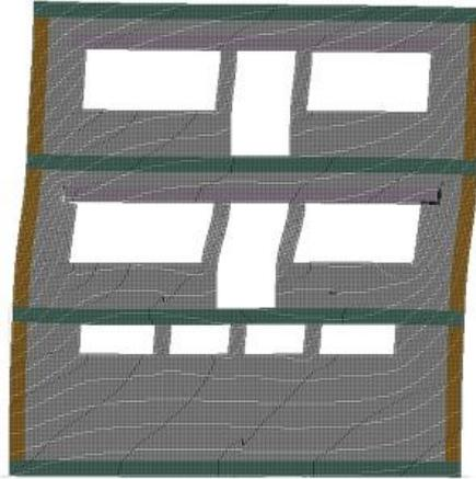
Figure 5: First form of vibration of the initially damaged model
