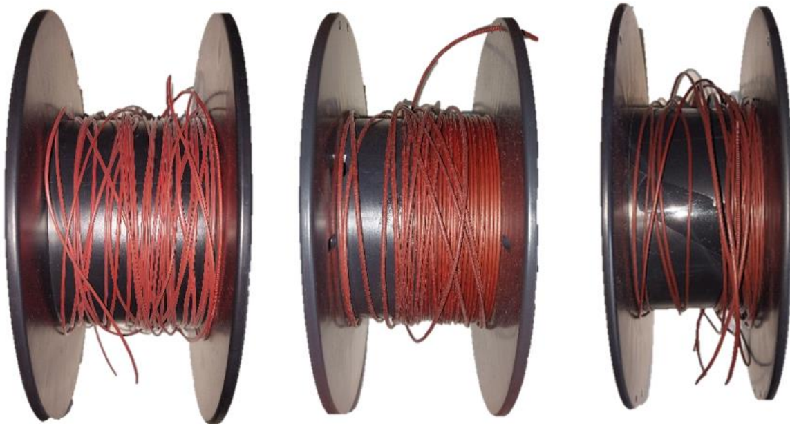
Figure 49 Piezoelectric composite filaments based on HDPE filled with: SbSI, SbSI/ \mu GC and SbSI/ s\mu GC
