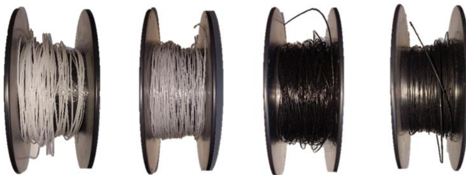
Figure 15 Examples of extruder filament, from left to right: HDPE, n\text{-Al}_2\text{O}_3 , \mu\text{GC} , s\mu\text{GC} .
