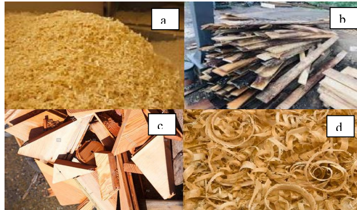
Fig 4. Residual biomass from the forestry industry, a. Sawdust, b. bark, c. Scrap wood, d. Wood chips/shavings
