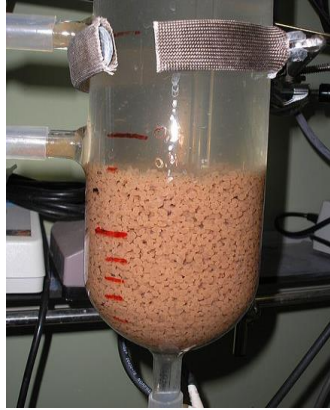
Fig. 6. Laboratory scale sequencing batch reactor [31]
