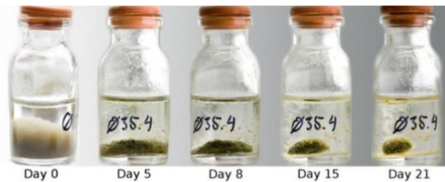
Fig. 7. A gradual progression of the photogranules under ‘‘static cultivation’’ [27]
