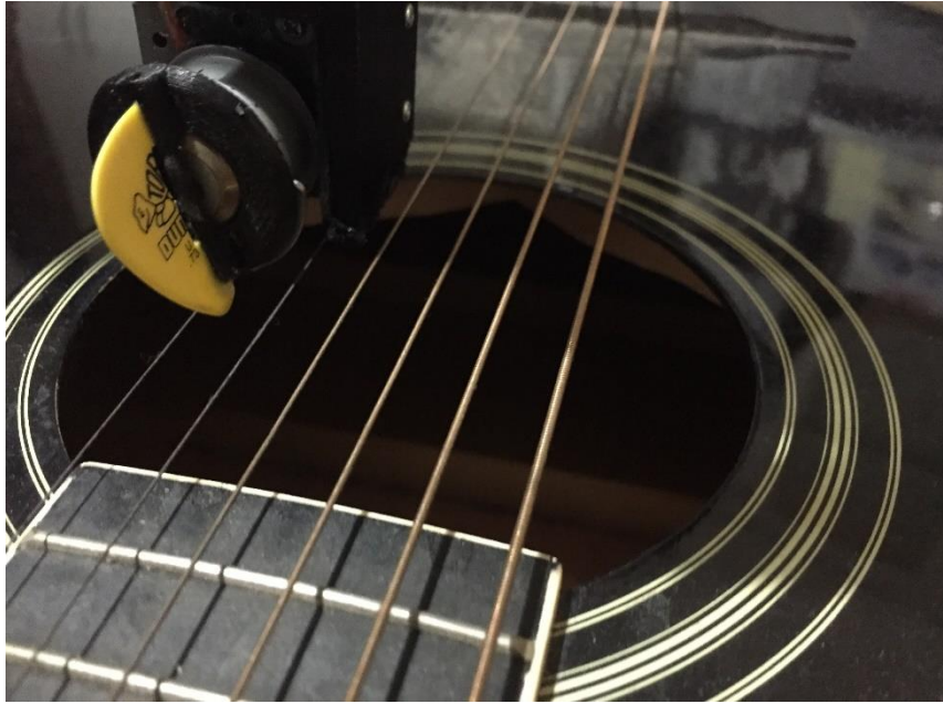
Fig. 12. Plucking mechanism based on a BLDC motor
