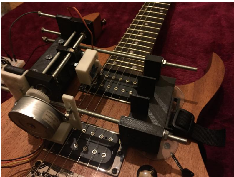
Fig. 9. Movable servo-based string plucking mechanism for electric guitars
